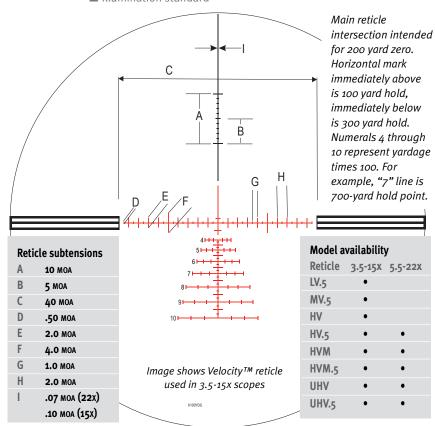
The Velocity 1000™ reticle is offered in several configurations, tailored to the ballistic profile of your load. The chart below shows each configuration's deviation, in minutes of angle, from a 200-yard zero point.
